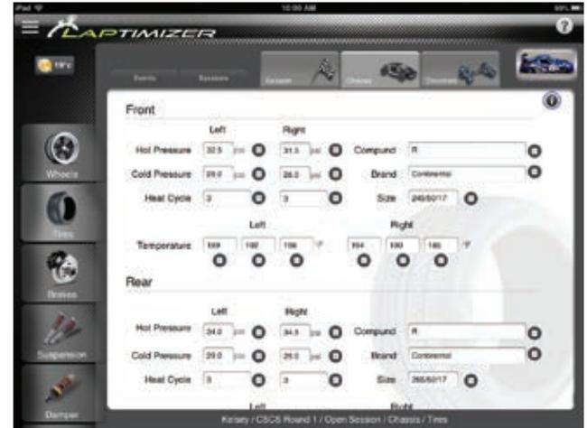
each session you run, which outlines the settings of all of the adjustable goodies your car has to play with. Things like pressures, spring rates, clicky damper knobs, anti-roll bar settings, brake pad compounds and fuel level would all be on your setup sheet. More advanced cars would also record wing angles, gear ratios, ride heights and the like. This is your input data. This is how the car will start the session.
